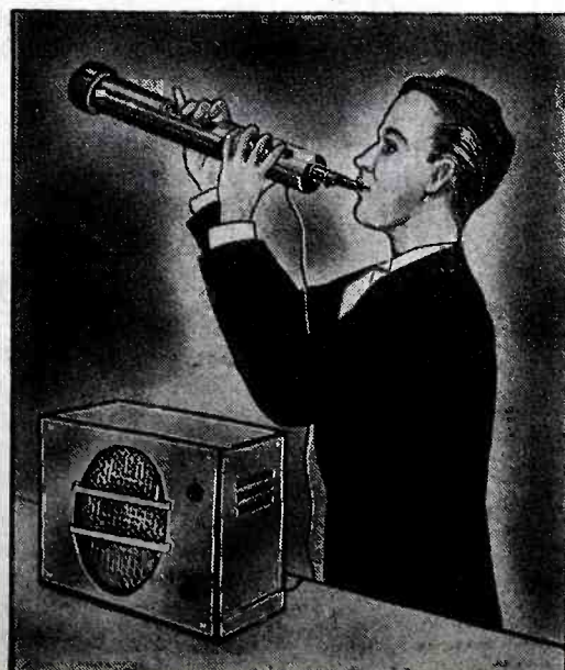
Fig. G. A felt plug permits the clarinetist's breath to escape, but absorbs the sound waves.
