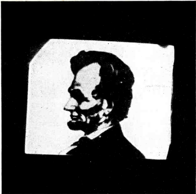
Fig. B. An unretouched photograph of the screen on the receiving tube.
