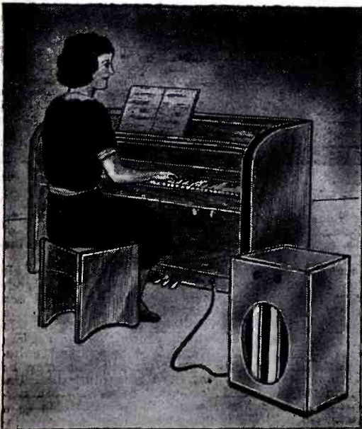
Fig. C. Ten times the volume of an ordinary concert piano is obtained without use of sounding-board.
