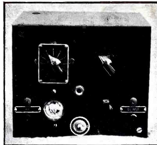
Fig. A. Front view of the neon tube test unit. Note the tube protruding from the panel.
